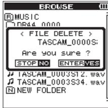
Press the **ENTER/MARK** button to delete the file, and press the **■/HOME** button to cancel the delete operation.
