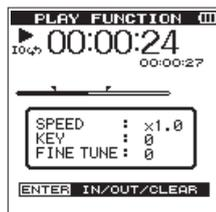
This position is set as OUT (end) point, and the unit will playback the section between the loop playback IN and OUT points.
