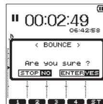
11. Press **ENTER/MARK** button to start track bounce and return to the Home screen after bouncing. Press the **■/HOME** button to return to the Home screen without track bouncing.
