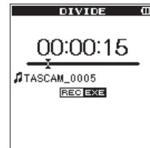
4. Use the **wheel** to determine the position where you want to divide the file and press **RECORD**.
