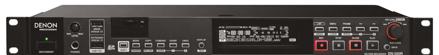
1RU DN-500R SD/USB Audio Recorder • Records to SD/SDHC and USB media in MP3 and WAV (up to 24-bit/96kHz) • Dual Record feature (records to both media options simultaneously for primary and backup recording) • Relay Record feature (continues recording to backup media when primary media is full) • XLR and RCA audio connections (analog and digital)
